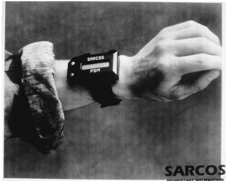
Figure 9.3. The Sarcos Personal Status Monitor System. The watchband is worn by the soldier. (Courtesy of S. Jacobsen, Sarcos, Inc., Salt Lake City.)
