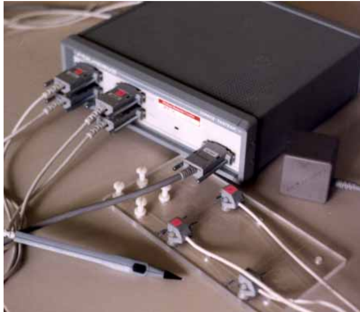
Figure 5.3. The Fastrack (Polhemus Navigation Science, Colchester, VT) controller box (background). In the foreground from left to right: stylus, three receivers mounted on a plate, and the transmitter.
