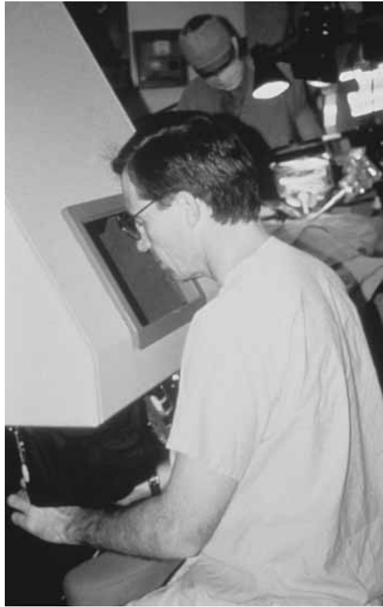
Figure 9.10. The surgeon's console on the telepresence surgery system—first generation. (Courtesy P. Green, SRI International, Menlo Park, CA.)
