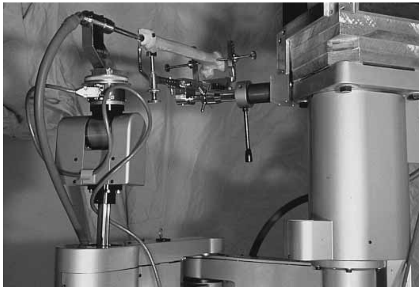
Figure 9.9. RoboDoc robotic surgery system for coring the femoral shaft in hip replacement. (Courtesy of H. Paul, University of California at Davis, Sacramento.)
