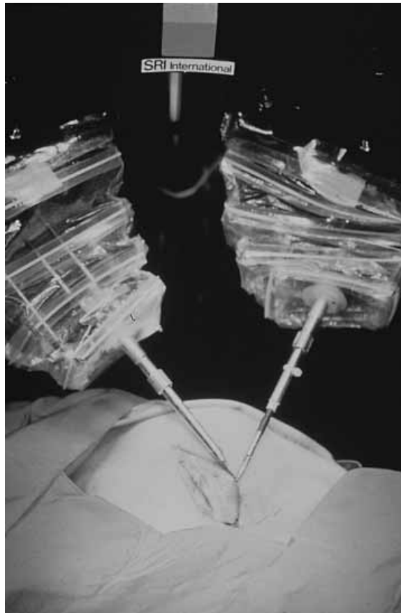
Figure 9.11. The remote manipulators of the telepresence surgery system—first generation. (Courtesy P. Green, SRI International, Menlo Park, CA.)
