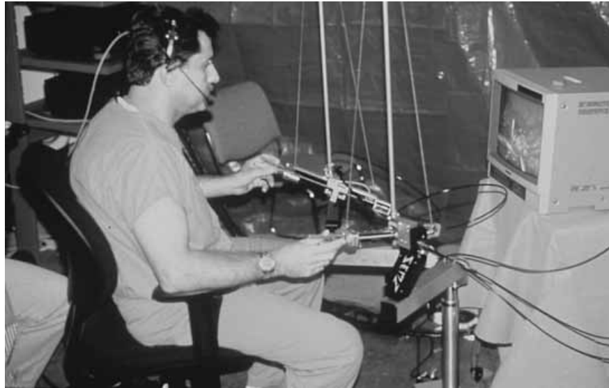
Figure 9.12. The Zeus Telepresence Surgery System. (Courtesy Y. Wang, Computer Motion, Inc., Goleta, CA.)
