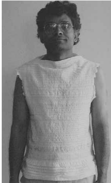
Figure 9.4. The Smart Tee-Shirt. showing fiberoptic and piezoelectric fibers woven into the garment. (Courtesy S. Jayaraman, Georgia Technology Institute, Atlanta.)
