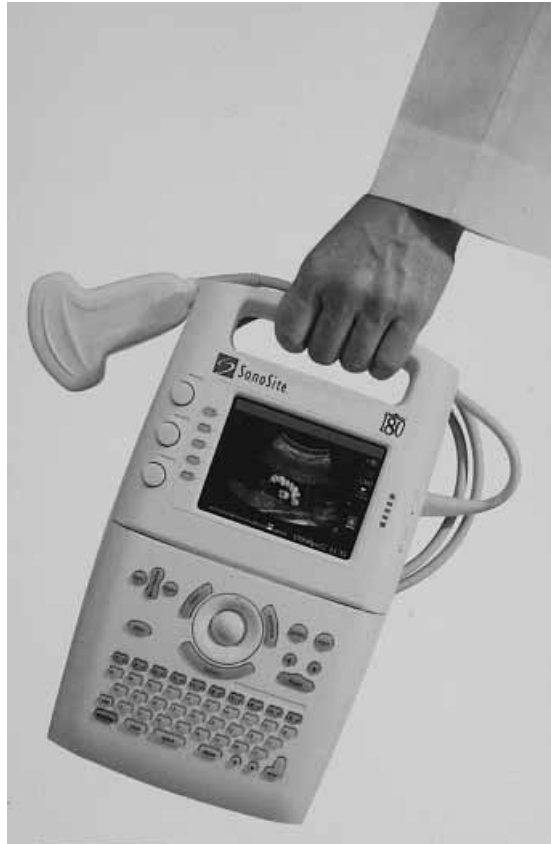
Figure 9.7. Small, handheld portable ultrasound unit by SonoSite. (Courtesy S. Carter, University of Washington, Seattle, WA.)
