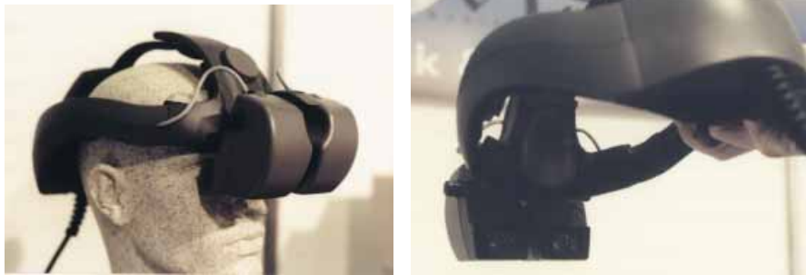
Figure 5.13. Prototype of the VISTA HMD. A , Side view. B , Inside view showing the two displays.
